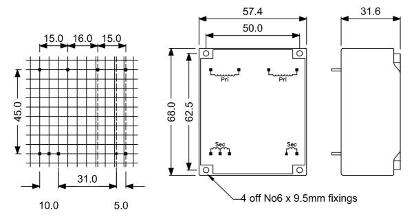
5mm pin grid PCB Pins 0.635mm sqr Pin length 5.0mm Hole size 1.0mm
